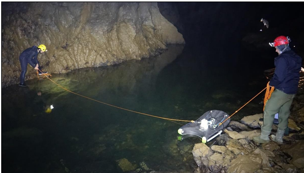
Figure 1. Stream profiling of the Pivka channel in the Planina Cave (photo: C. Mayaud).
